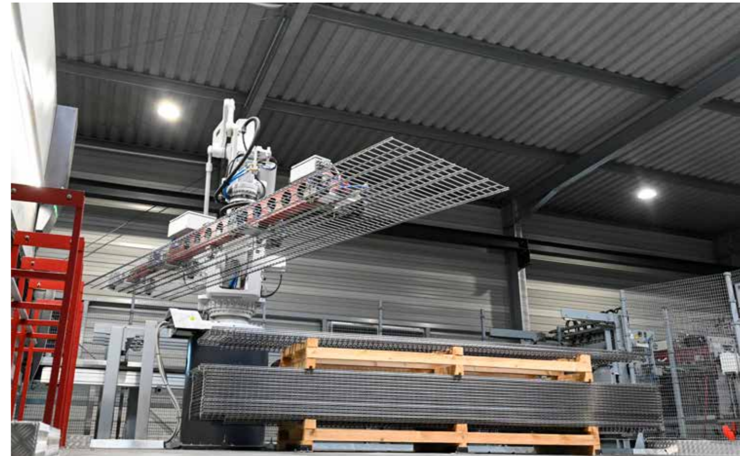
Automated removal of the finished steel mesh mat
